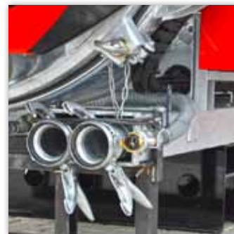
Integrated forklift tubes; ideal for hose storage
