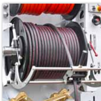
Hydraulic drive for HP reel with e.g. extendable layered hose guiding system
