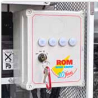
Control box in motor/pump combination
