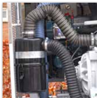
Combined oil separator / silencer (V-140/60 model)
