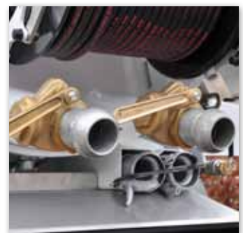
Discharge valve + Suction valve
