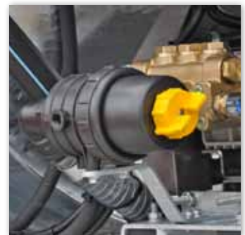
Automatically closing water filter with rinsable element
