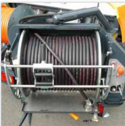
Rotating stainless steel drip tray prevents your machine from becoming dirty
