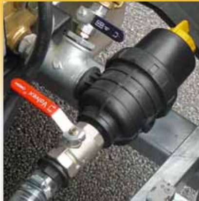
Water filter (PE) with automatic stop valve
