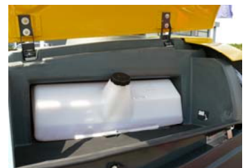
TANK FOR SOAP STORAGE
