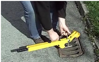
1: Slot T-Key Between Slats and Tighten
