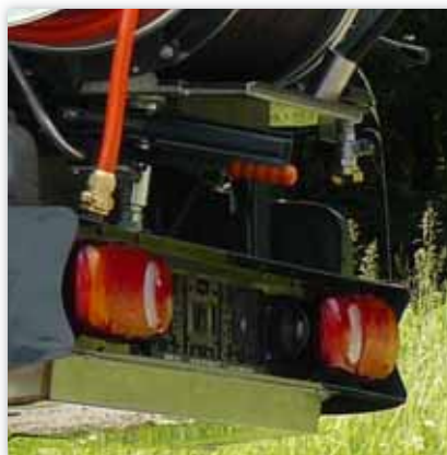
Integrated lighting units, protected in the bumper
