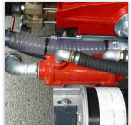
Reliable engine temperature management by means of a heat exchanger (diesel version)
