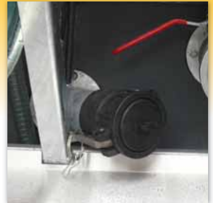
Fixed ventury-type ejector for filling the tank with surface water
