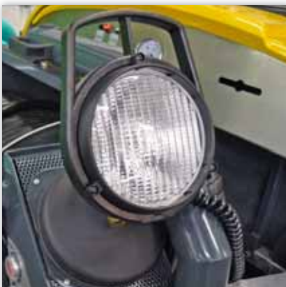
Working light with magnetic bracket
