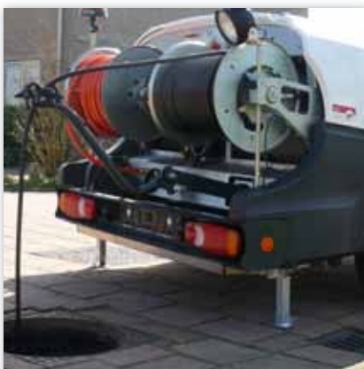
Advanced hose guiding system with fold-out operating arm (optional)
