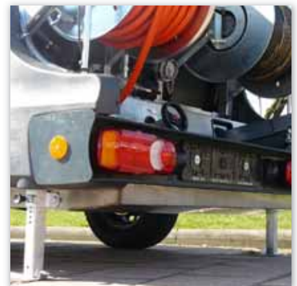
Support legs with quick adjustment; extra security for hydraulic reeling of the HP hose (supplied with hydraulic version)
