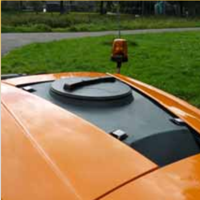
Polyethylene water tank; cover with snap-lock seal
