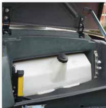
Transparent fuel tank with handy filling option
