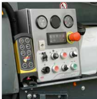
Different operating boxes including electronics attuned to petrol/ diesel version: mounted in lockable, vandalism- and water resistant toolbox
