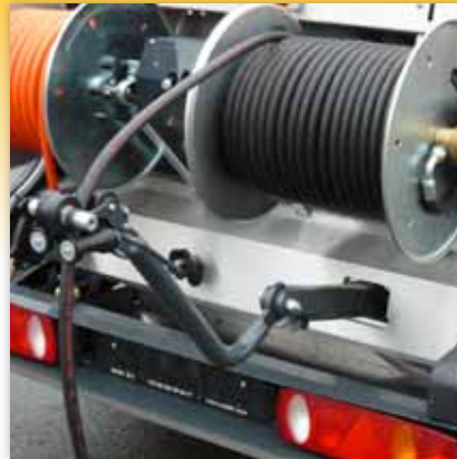
Hose guiding system with fold-out operating arm
