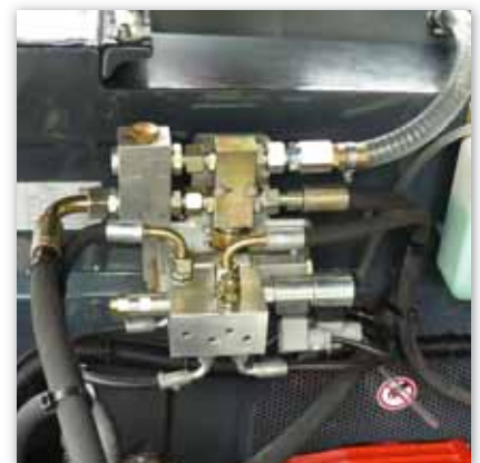
Minimum valve wear due to the unique 2x2 hydraulically operated pressure on/pressure off system (diesel version in combination with hydraulically driven HP reel)
