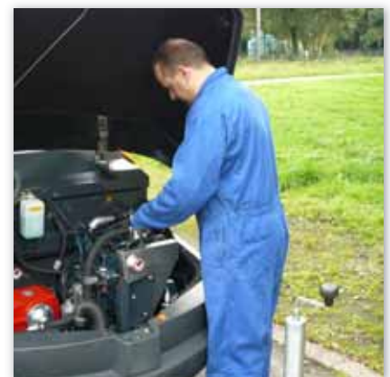
Lockable bonnet with large opening angle; ideal for service and maintenance of engine/ pump compartment
