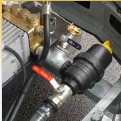
Waterfilter (PE) with automatic water stop
